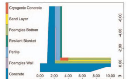
Figure 6: Wall to slab connection and thermal corner protection TCP
