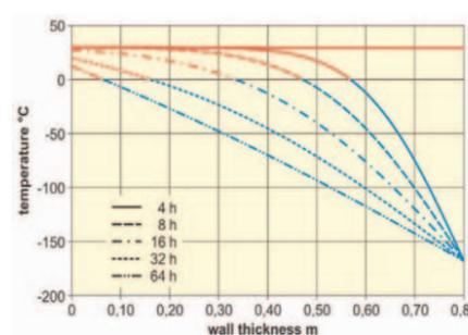
Figure 2: Temperature in the wall at 4, 8, 16, 32 and 64 hours
