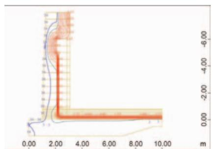
Figure 7: Isothermal curves in the wall to slab connection and thermal corner protection
