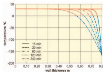
Figure 1: Temperature in the wall at 15, 30, 60, 120 and 240 minutes
